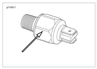
Figure 1. Rear Stop Light Switch Identification: Sharp Edges Are Gone On New Switch
